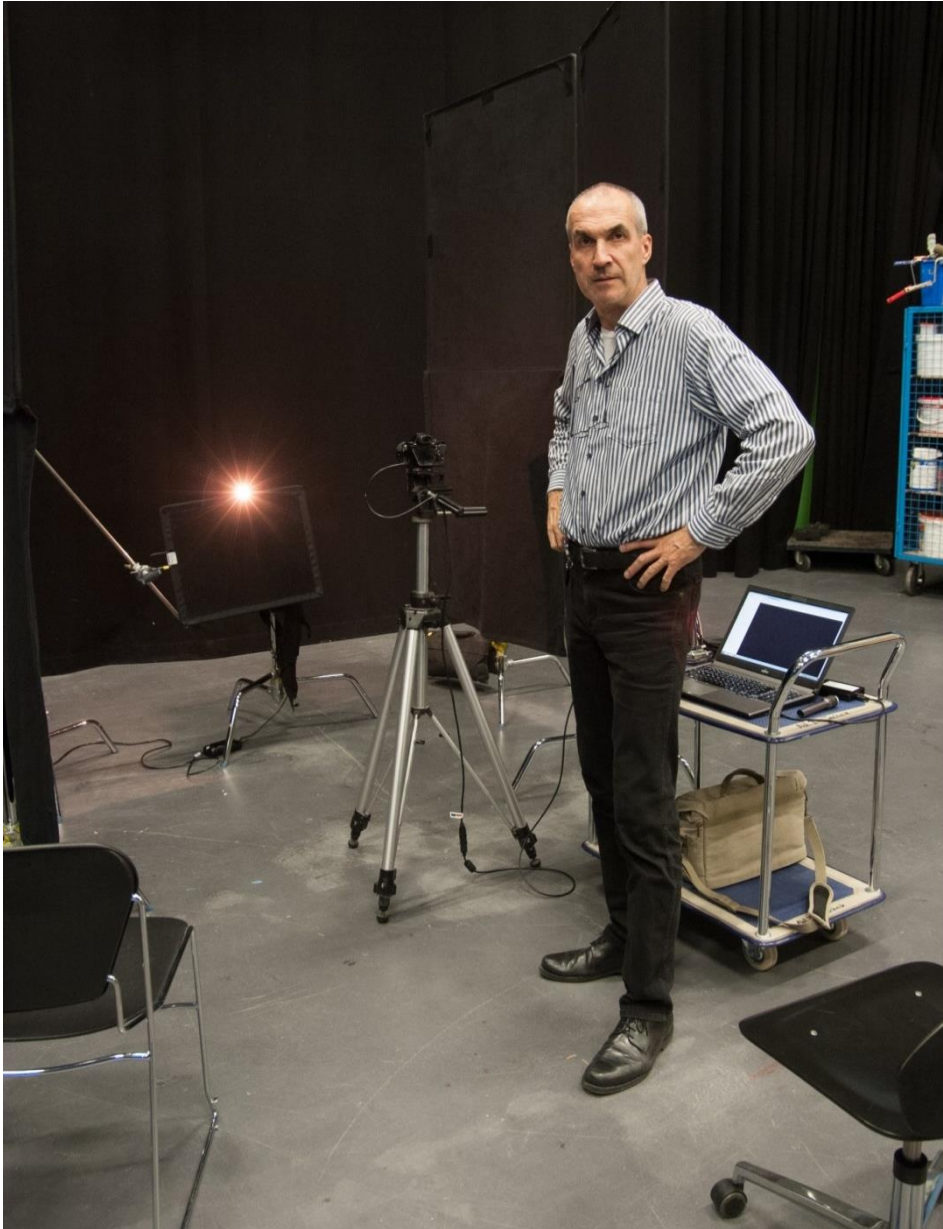
Fig 5: Peter C. Slansky with the test setup in the TV studio 1 of the University of Television and Film Munich. The Sony a7S camera with the Canon FD 1.4/50mm lens is pointed to the tungsten bulb (point shape light source). The alternative areal light source, a LED torch with a white calotte, lays on the trolley right from the laptop. For the real tests the other studio lights were switched off completely. Photo by Bernd Gahrken.
