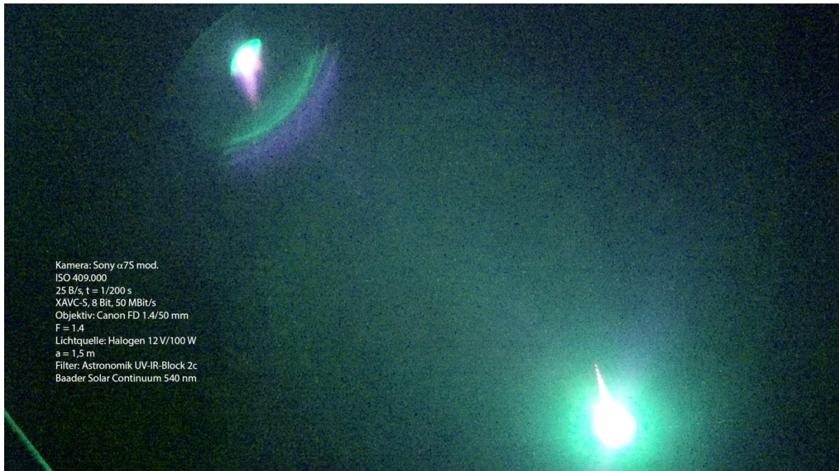
Fig. 8: Point light source narrow band filter 540 nm at 1000 times overexposure: There is a clipped area of the same size as for the terminal flash in the video but around it there is a very wide green halo. Also, there are
