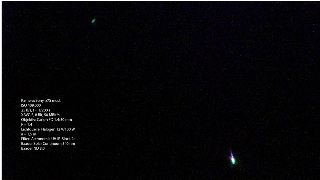
Fig 7: Point light source with narrow band filter 540 nm at normal exposure: The only artefact is a small green flare because of the narrow band filter in front of the lens.
