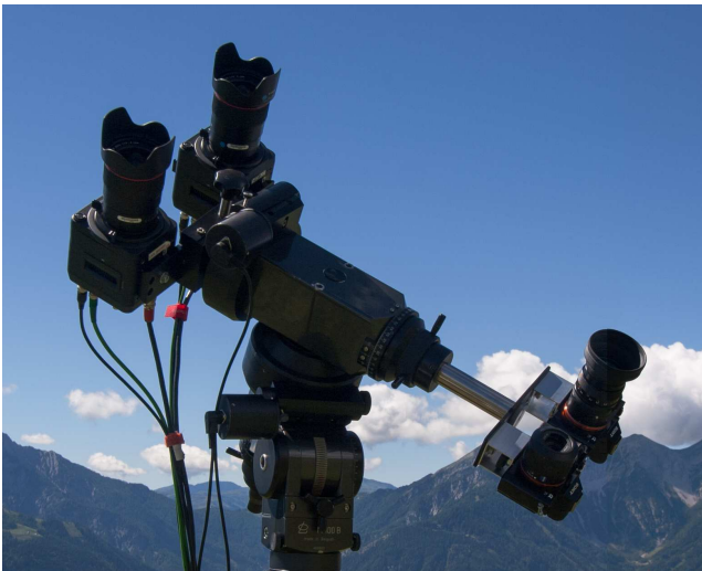
Figure 6 – Instrumentation for the 2016 Perseids, Figures 5, 7 and 8. Two Canon ME20F-SH cameras and two Sony \alpha 7S were mounted on a Lichtenknecker M 100 B, with an image field rotating around the sky North Pole. The location is Emberger Alm in the Austrian Alpine Mountains, 1760 m above sea level. On the bottom of the mounting (not in the picture) two data recorders were connected to the Canon ME20 cameras. Over all, ten AC power supplies were needed.
