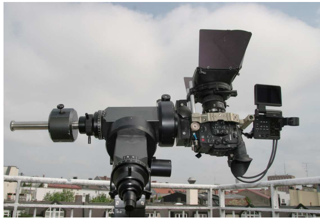
Figure 2 – The instrumentation for the Camelopardalid 2014 May 24, 01 h 58 m 08 s UTC, Figures 1 and 3 was a Canon EOS C 300 with a Zeiss Cine Superspeed Distagon 1.2/18mm on a Lichtenknecker M 100 B mounting on my rooftop terrace in the Munich city center, Germany.
